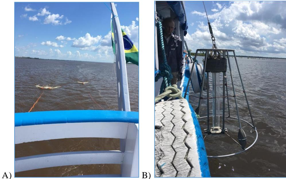
**Figure 1** – (A) Seismic equipment in acquisition and (B) Coring equipment being deployed, both from Samara Lopes XII vessel.
