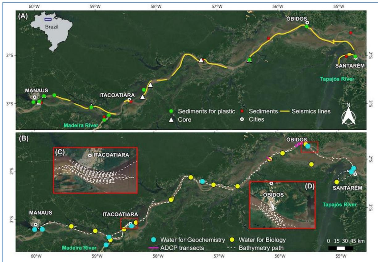
**Figure 2** – Map of Data Acquisition : showing location of geophysical data, water and sediment samples acquired on the SAMARA Lopes XII boat during AMANAUS cruise, July 2023.
