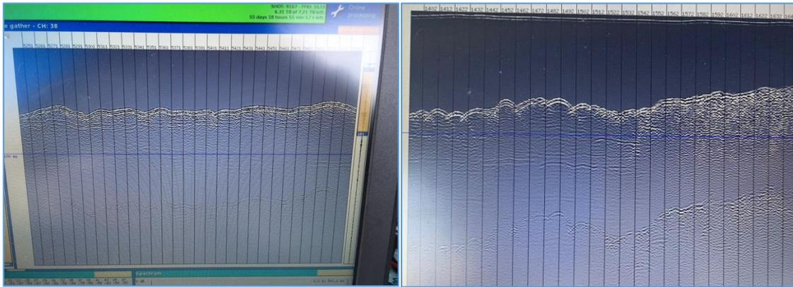
**Figure 5** - Preliminary results of not processed seismic data showing (A) giant dunes and (B) abrupt contact between Sandy/Rocky river-floor
