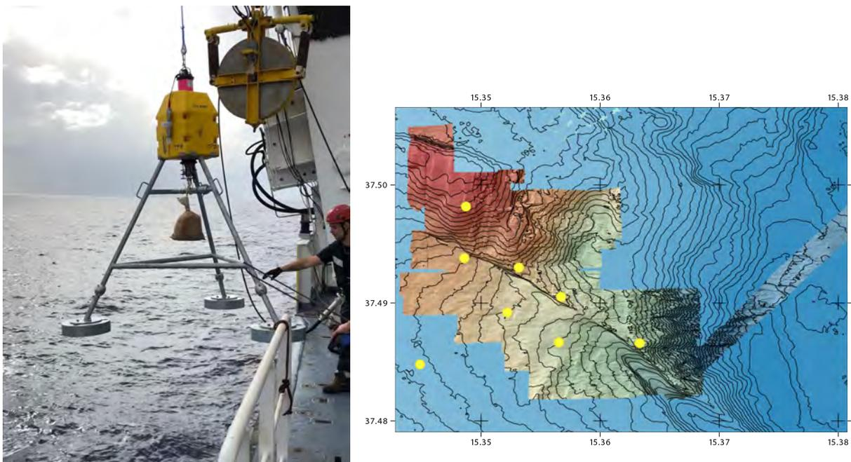
*Figure 10: (left) deployment of a sea-floor geodetic station, with Canopus acoustic beacon (the pink cylinder visible at the top), buoyancy (yellow polyhedral cover) and the metallic tripod; (right) map of study area, with the micro-bathymetric data (ROV Victor6000) and showing the location of the 8 sea-floor geodetic stations deployed (yellow circles), 4 to the north of the fault, and 4 to the south.*
