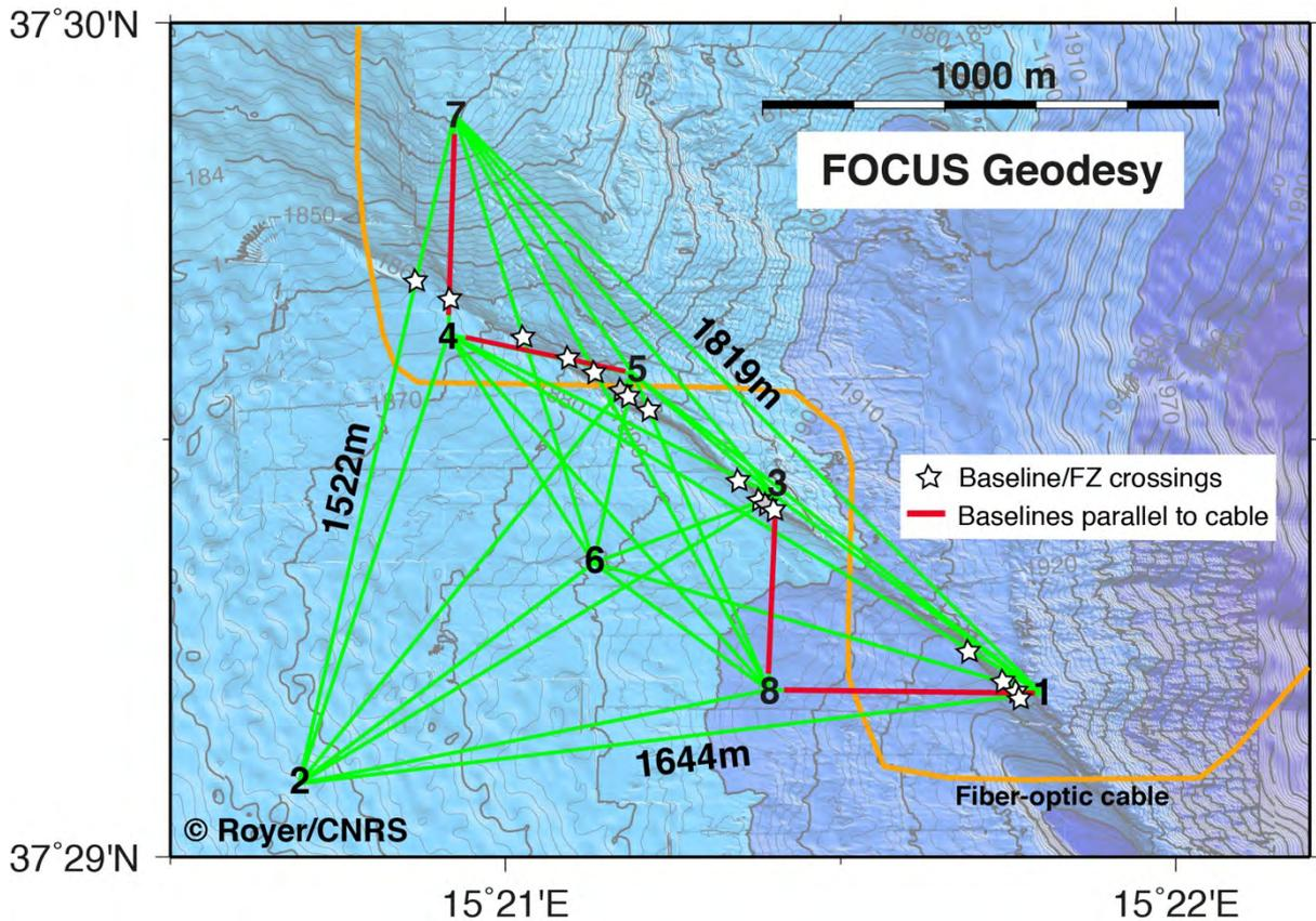
Figure G1: Geodetic beacons (numbers) and baselines (green lines). Stars show the crossings between the North Alfeo fault and the baselines. Red lines show the baselines parallel to the fiber-optic cable, which will be used to calibrate the displacements measured by BOTDR.
