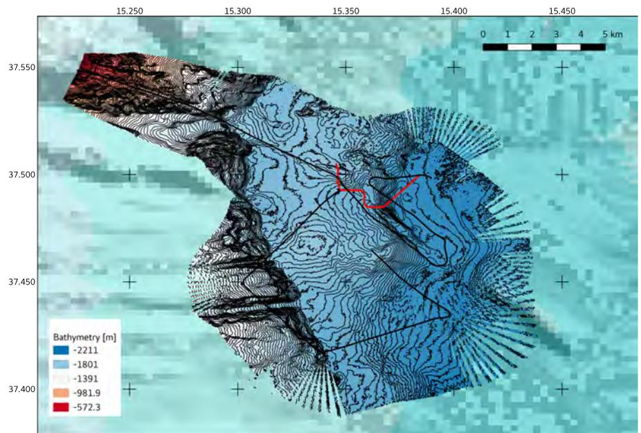
**Microbathymetry data acquired with the ROV Victor 6000**
