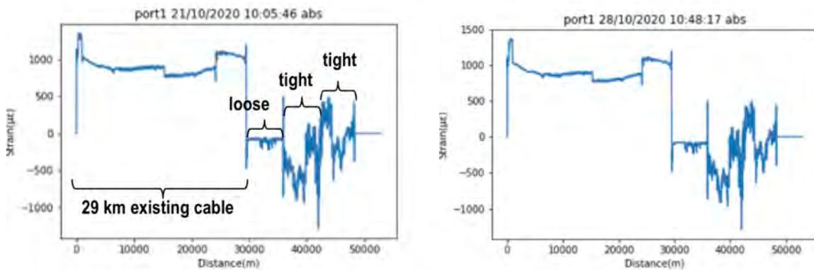
Fig. 15: (left) BOTDR absolute baseline (acquired on 21 Oct. 2020, 3 days after cable deployment); (right) BOTDR absolute baseline (acquired on 28 Oct. 2020 after installing new software on VIAMI interrogator), There is no discernible difference between the two measurements.
