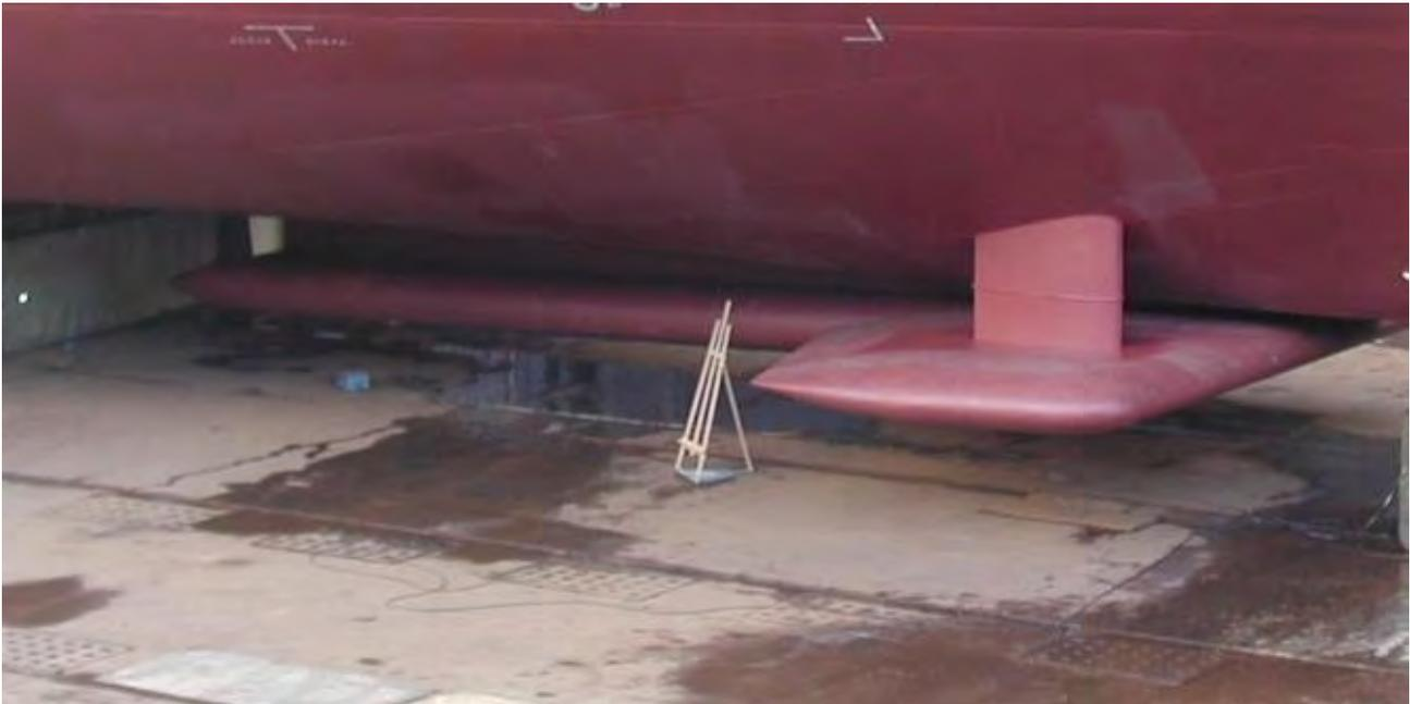
*Figure B1: The RESON Seabat7150 multi-beam echo-sounder at the Pourquoi Pas.*
