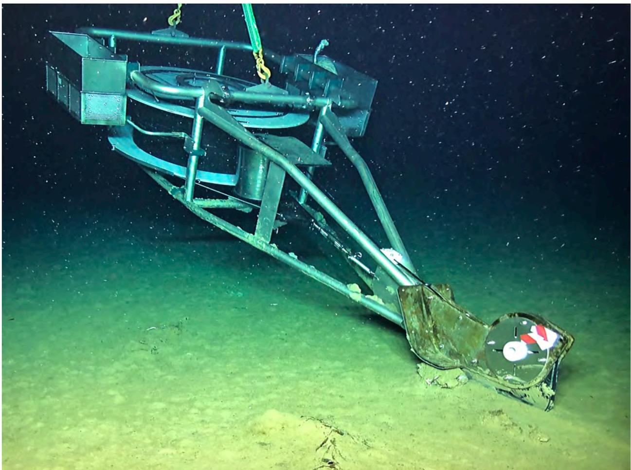
Figure 12: Deep Sea Net plow (model 2020) on the seafloor. Most of the 6.2 km long fiber-optic cable can be seen, spooled on the reel (drum).
