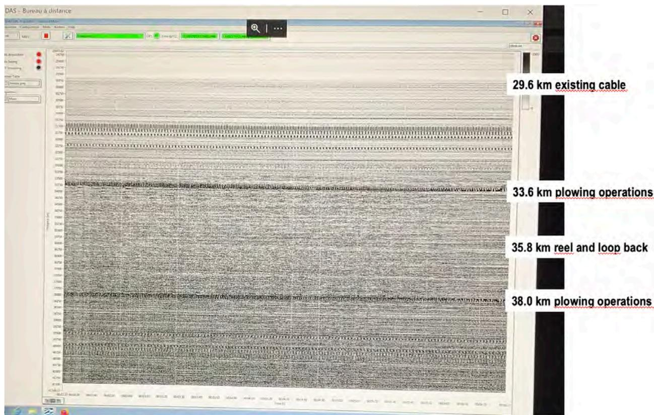
Fig 17: DAS acquisition during FocusX1 cable deployment operations on 17 Oct. 2020. 4 km of cable have been deployed and 2.2 km are still on the reel / drum. Strong oscillations are observed between km 31 and 32 (and the same are observed on the return loop around km 40 to 42).
