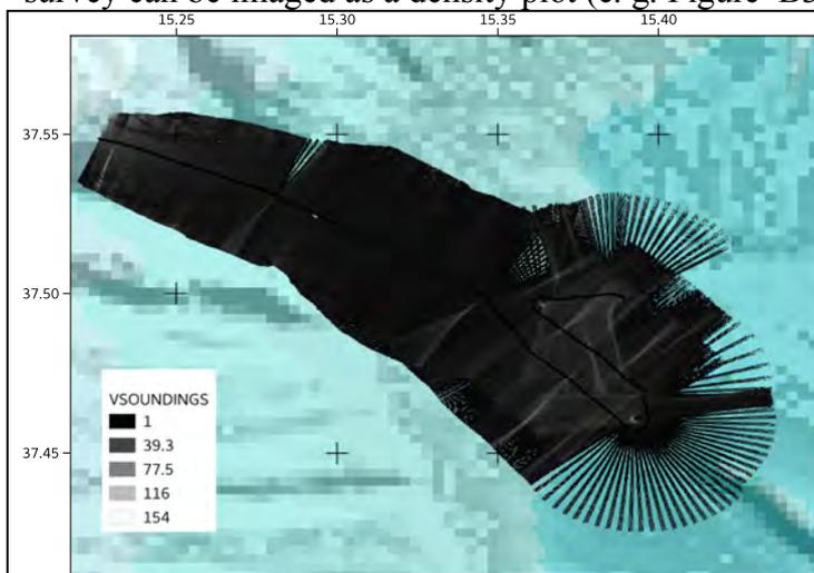
Figure B3: Depth sounding density for the ship-hull survey.
