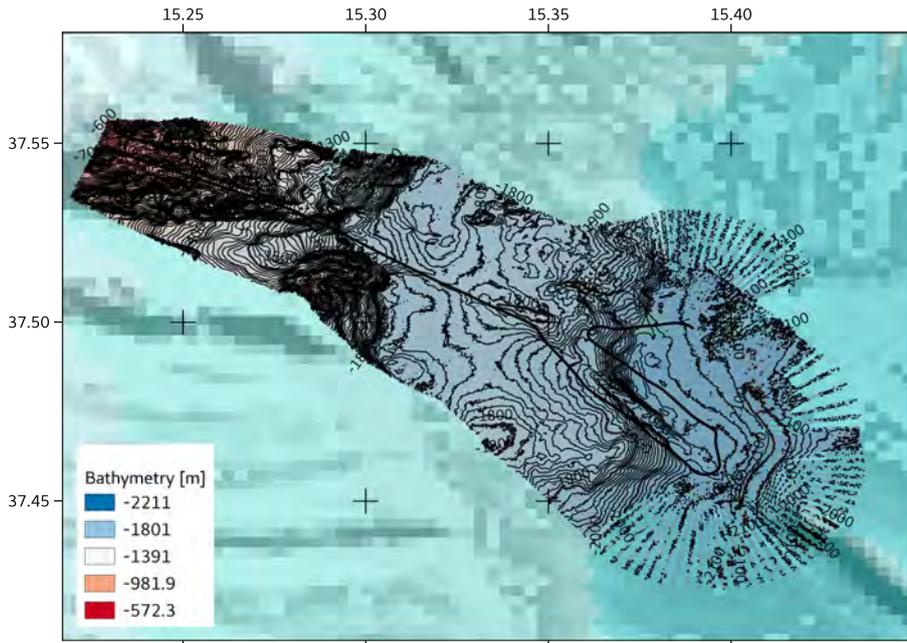
Figure B4: Seafloor bathymetry of the study region from the hull mounted RESON Seabat7150 multi-beam echo-sounder in survey 1..
