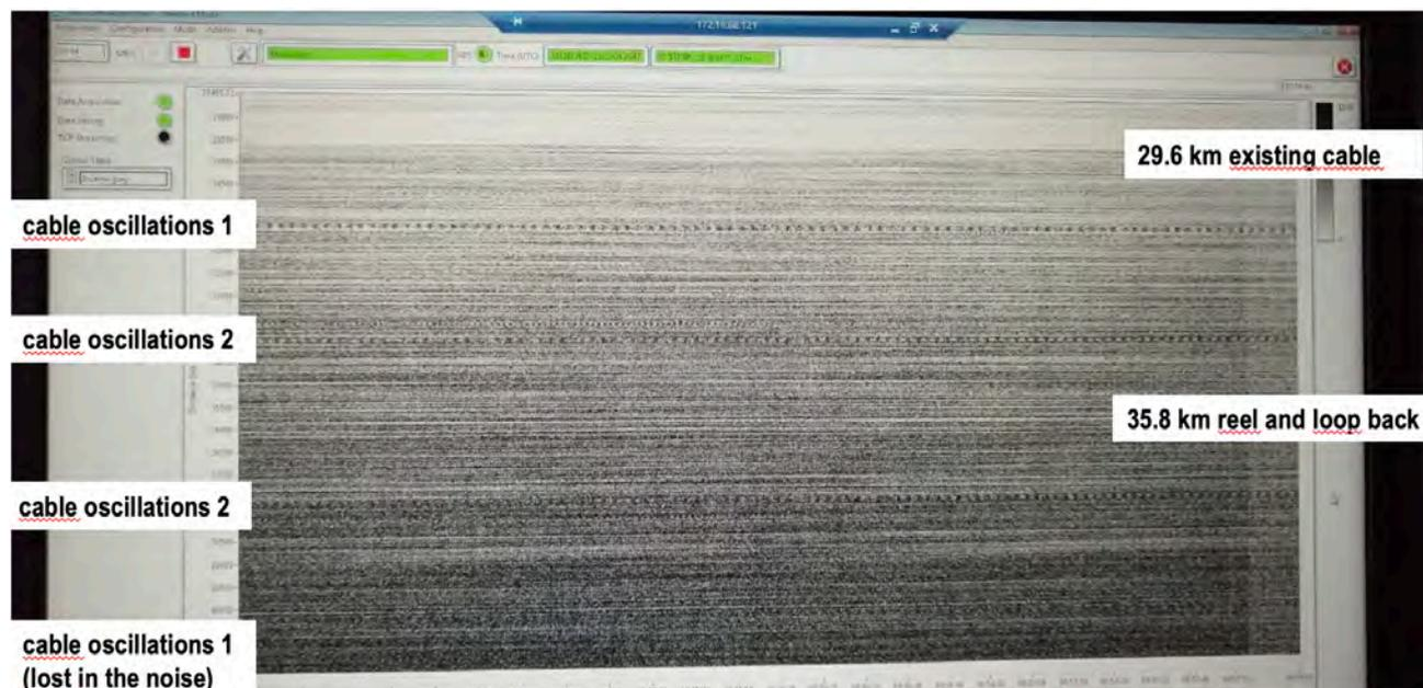
Fig 18: DAS acquisition from 21 Oct. 2020, 3 days after FocusX1 cable deployment operations were completed (on 18 Oct.). Note the symmetric oscillations due to the fiber path out to and back from the plow drum (located at 35.8 km distance from the port laboratory of INFN-LNS in Catania). Noise levels increase significantly beyond 40 km distance.
