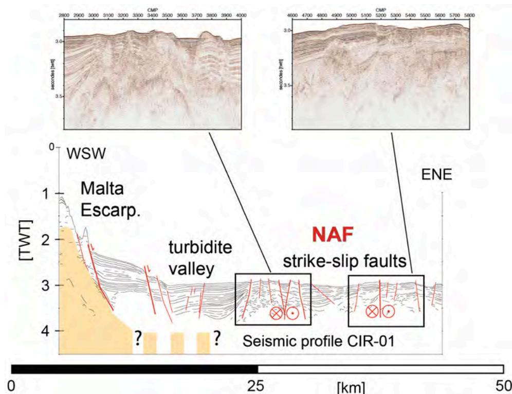
Figure 4: Seismic profile CIR-1, with a line drawing (below) and close-up of zones cross-cut by strike-slip faults (Gutscher et al., 2016). NAF = North Alfeo Fault. For location see Fig. 2A.
