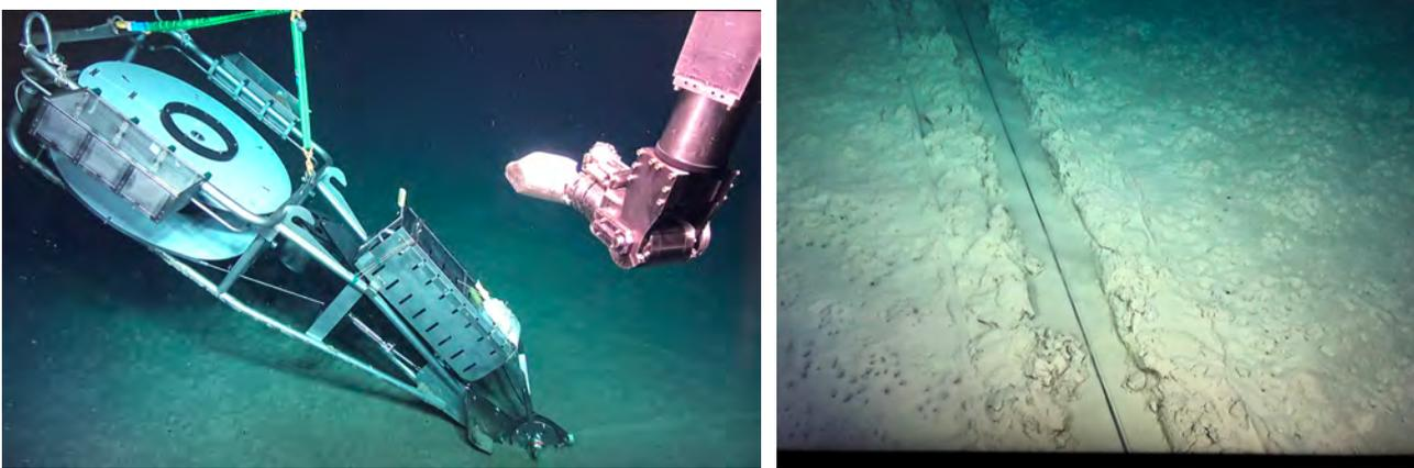
*Figure 8: (left) Deep-sea net plow (version 2020) on seafloor during tests on 3 March 2020 offshore Toulon in 680m water depth, with dummy cable-end module (CEM) and ROV arm; (right) plow track with groove (mini-trench) showing successful burial of cable (a test length of 500m was deployed and buried)*
