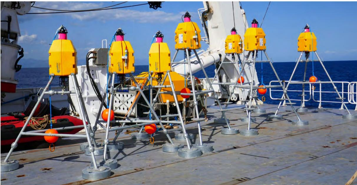
Figure G2: Geodetic beacon setup: each acoustic beacon is mounted on a 2.5m- or 3.0m-high tripod above the seafloor (Figure 3). The beacons are equipped with an external temperature sensor (fixed on the yellow floats).
