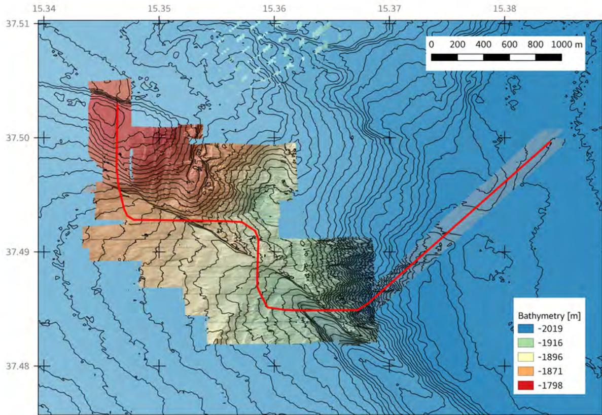
Figure B7: Seafloor microbathymetry from the ROV dives. Resolution of the grid is 2m and contouring every 5m. Red line depicts the provisional cable location.
