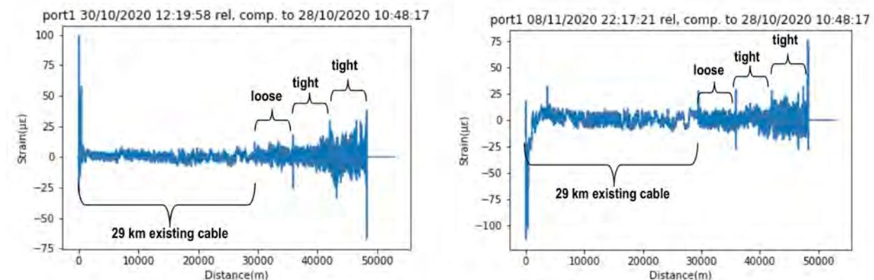
Fig. 16: (left) BOTDR relative strain measured on 30 Oct. (compared to 28 Oct. baseline) along the entire 48 km optical path; (right) BOTDR relative strain measured on 8 Nov. (compared to 28 Oct. baseline) along the entire 48 km optical path. The noise level is about  $\pm 5$ -10 microdefgs for the loose fiber, and about  $\pm 10$ -20 microdefgs for the tightly bound fibers, increasing progressively beyond 40km distance.
