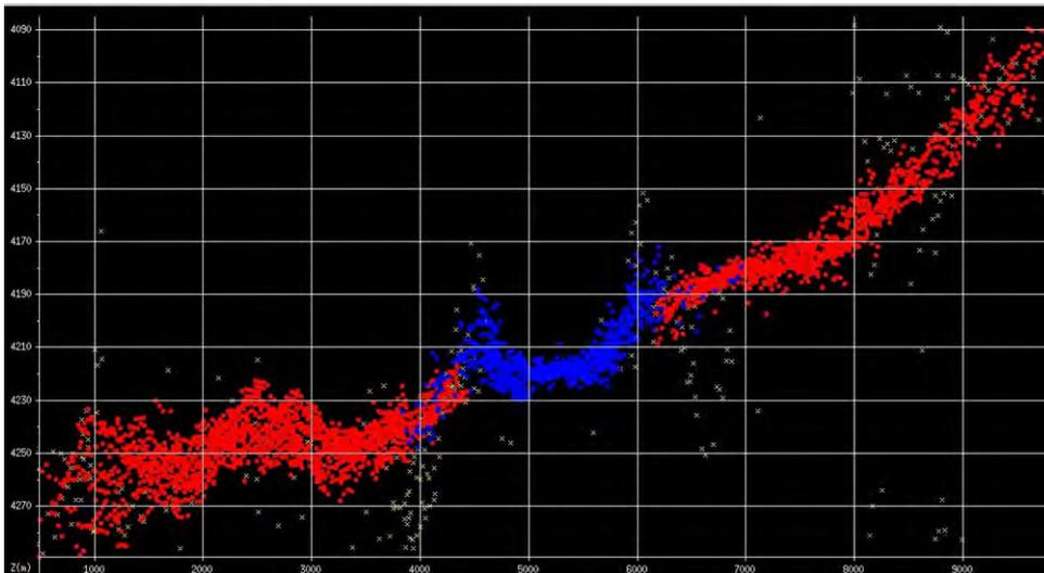
Figure B2: Profile of all beams from one signal perpendicular to the ships route. Gray points are outliers which are automatically excluded during the acquisition. The difference between blue echos (amplitude detection) and red echos (zero-phase detection) is cleaned manually. The larger variability of the outer echos is due to the decreased resolution of the outer beams.
