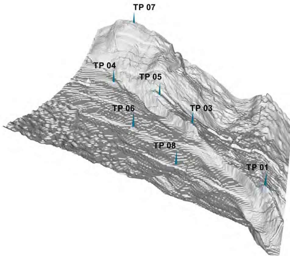
Figure 8: Seafloor microbathymetry (3-D view) from the ROV dives with the location of the geodetic stations.
