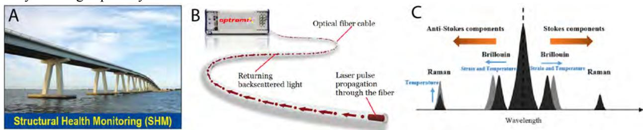
Figure 7: Large-scale infrastructures and BOTDR monitoring, A: SHM - example of bridge, B: Principle of backscattering and BOTDR, C: Types of backscattering during laser reflectometry (Rayleigh - central peak, Brillouin and Raman). The Brillouin spectrum of a given fiber shifts as a function of temperature and strain.
