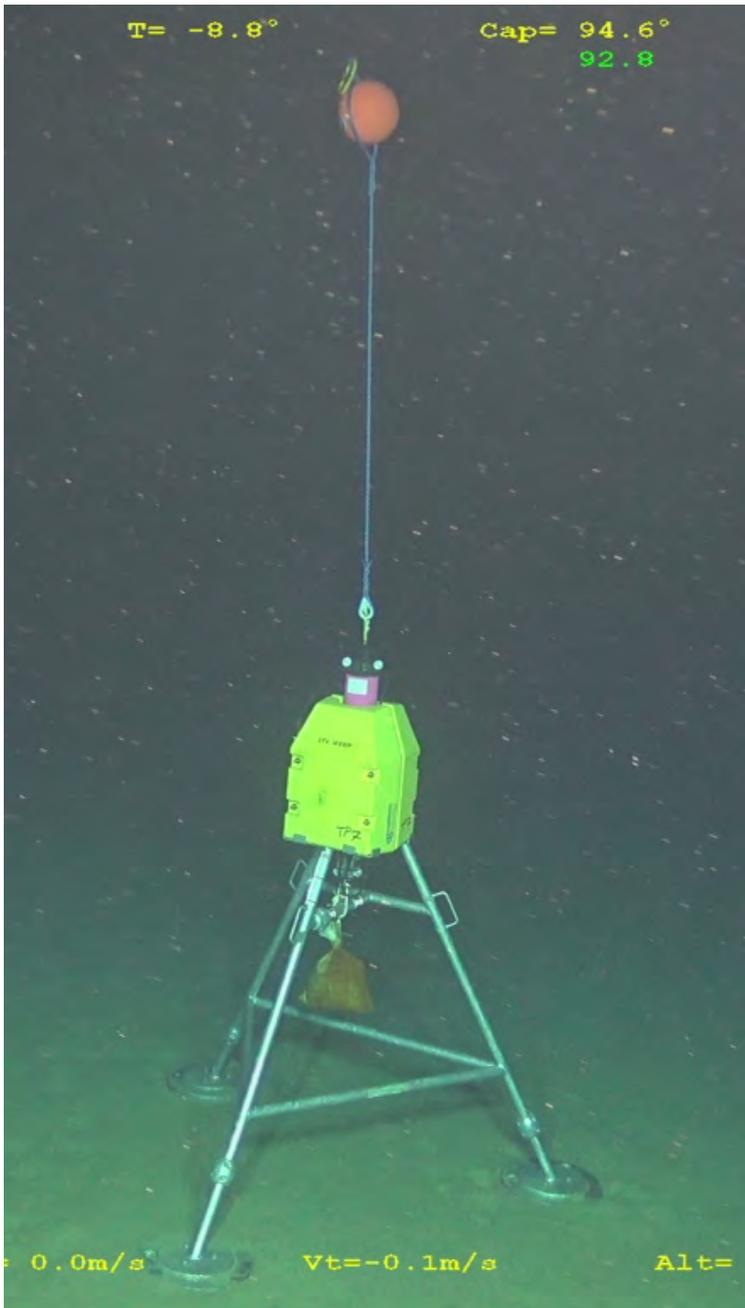
Figure G3: One of the beacons laid on the seafloor, inspected by ROV Victor. Sites with smooth bathymetry were selected.
